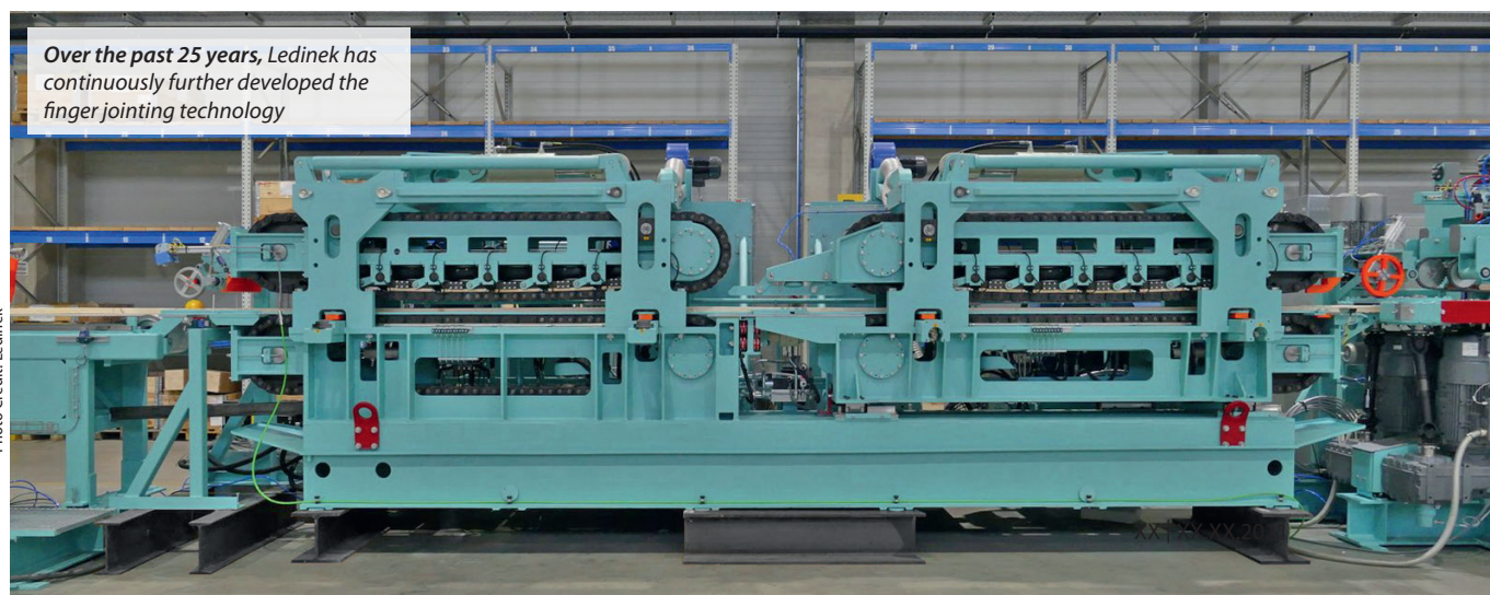
With an output of up to 40,000 meters per shift, the Kontizink 5000 is the most powerful of Ledinek's finger jointing machines
